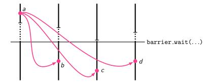
Accesses before (a) and after (b, c and d) the barrier cannot execute simultaneously. There is <u>no</u> data-race.
