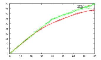
Wallclock times are divided by the running time of our faster sequential implementation: ./fast.out -d3 18. SP80 is the "parallel" implementation, ST80 is the pthreads implementation.
