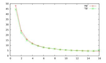
Wall clock time in sec. P8 is the "parallel" implementation, T8 is the pthreads implementation.
