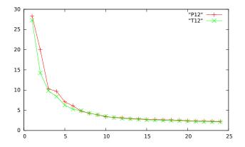
Wall clock time in sec. P12 is the "parallel" implementation, T12 is the pthreads implementation.
