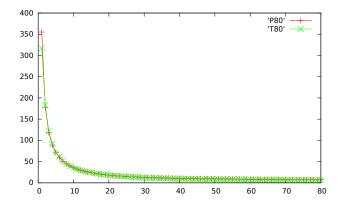
Wall clock time in sec. P80 is the "parallel" implementation, T80 is the pthreads implementation.
